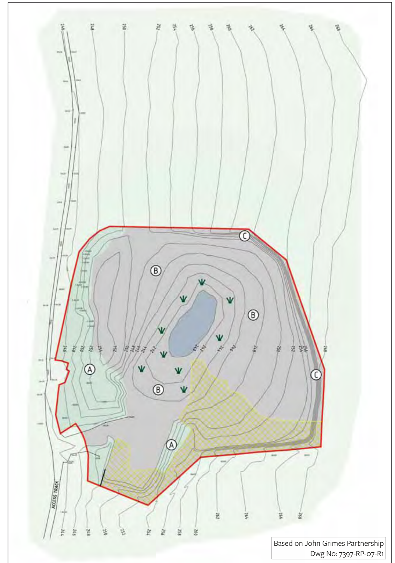
Figure 16: Restoration Proposals for Existing Permission
